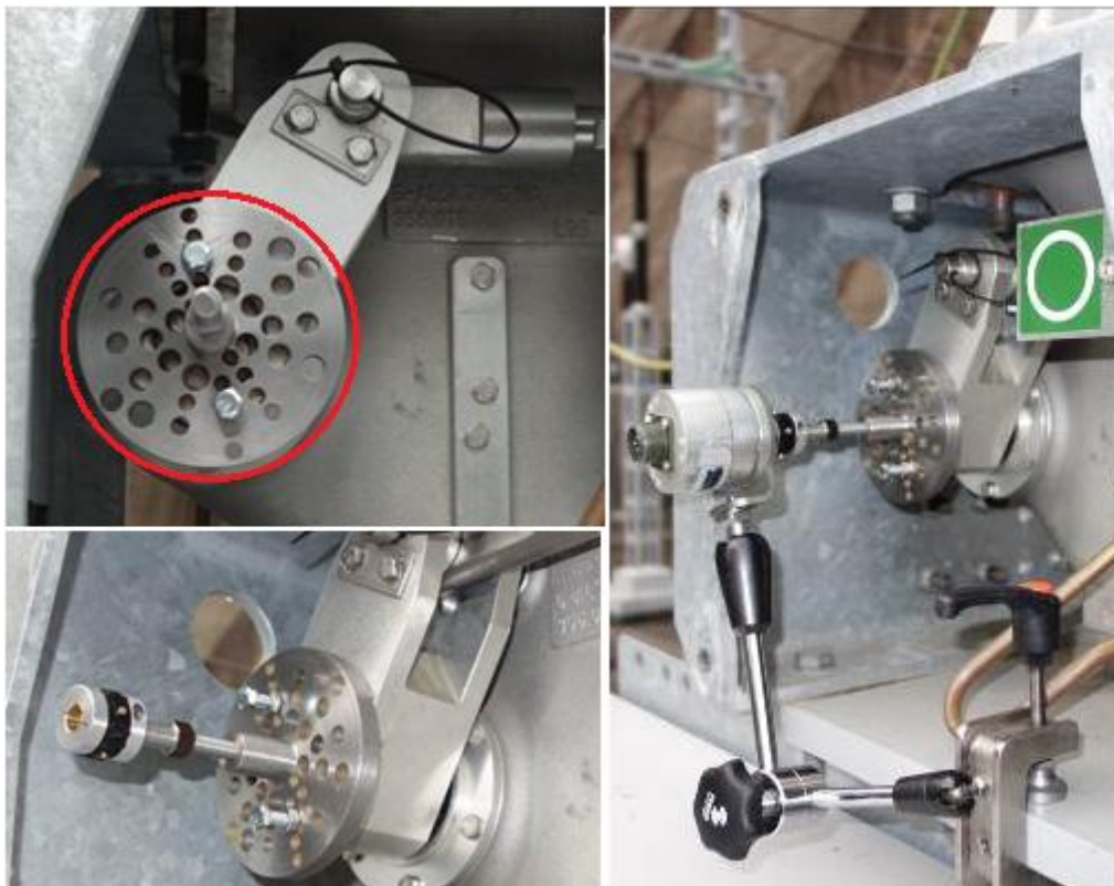
Figure 11. Installation of rotary (digital) transducer in the SIEMENS 245 kV CB. type 3AP1 FI using universal adapter for rotary transducer mounting
